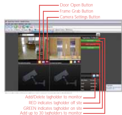
Visual door control with 2 active cameras, monitoring 3 cameras
