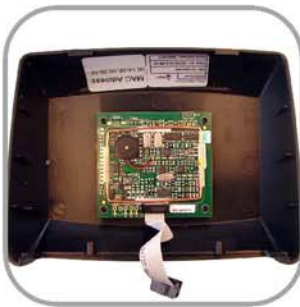
Tag Reader Coil mounted behind the screen
